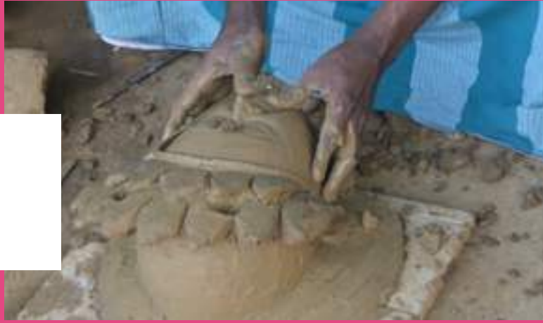
Preparation of clay mould
