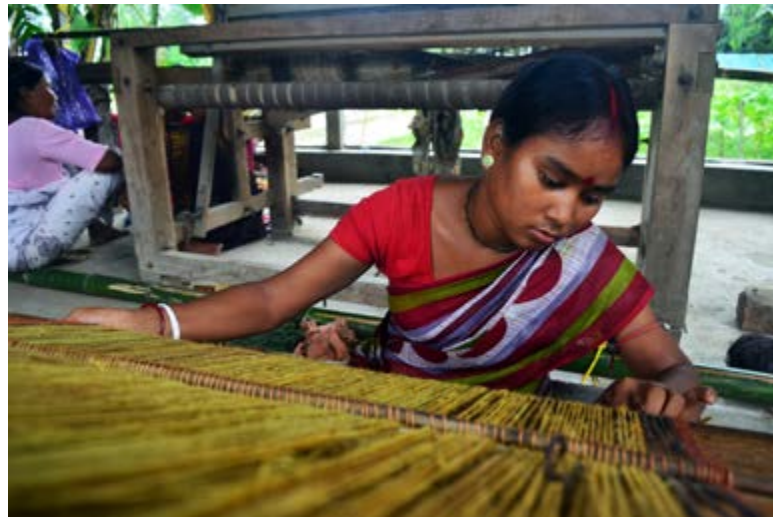
Dhokra weaving process (Above, left and centre) Drying and dyeing jute yarns (Above right) Arranging the jute strips in the spindle to give it a finer touch (Below left) Setting the fine jute strips in the loom (Below right) Weaving the jute strips in back-strap loom
