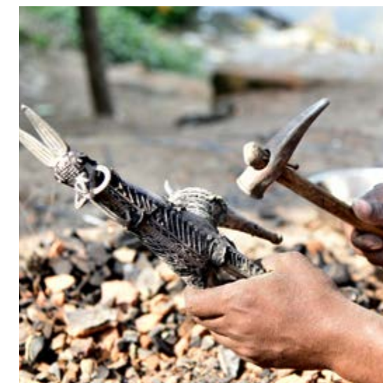
Dokra crafting process (Above left) Handcrafting designs on clay model with wax and resin (Above right) Creating the mould (Centre left) Filling the mould with metal (Centre right) Putting the mould in furnace (Below left) Breaking the mould after taking it out of the furnace to get the metal product (Below right) Polishing the finished product
